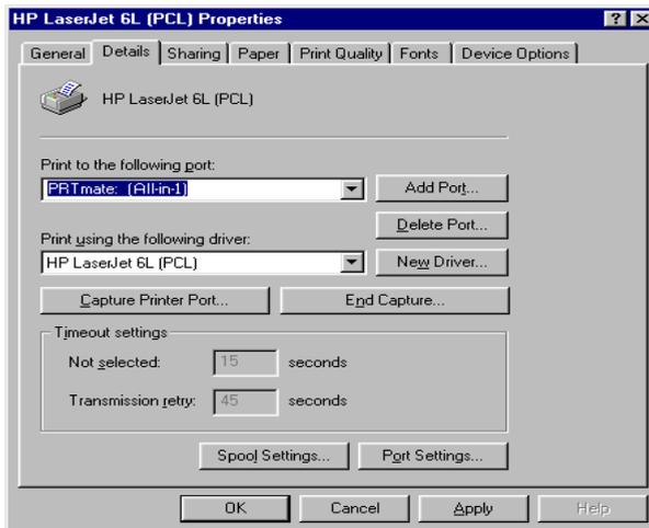
3. Choose the "PRTmate: (All-in-1)" from the list attached under the *Print To* item. Be sure that the *Printer Driver* item is configured to the correct driver of your *server*
