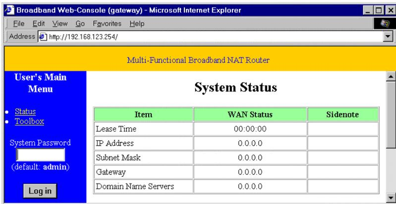
Activate your browser, and *disable the proxy* or *add the IP address of the SMC7004BR into the exceptions*. Then type this product's IP address in the *Location* (for Netscape) or *Address* (for Explorer) field and press ENTER. For example: *http://192.168.123.254*.
